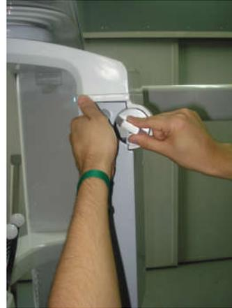
2. Rotate the knob 180 degrees until you lock the sensor
