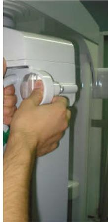
In order to change from Cephalometric to Panoramic mode, push the locking button close to the panoramic sensor in C-arm. The equipment will automatically change the configuration to Panoramic mode.
