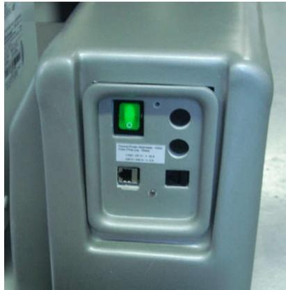
When the main switch is turned on, the machine will perform a self-check. If everything is within specifications, the display will show the x-ray counter.
