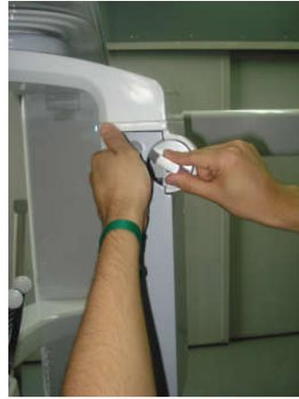
1. Hold the sensor tightly with your left hand and push the locking button with your right hand.
