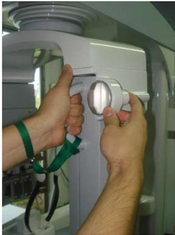
3. Hold the sensor tightly with your left hand and push the locking button with your right hand
