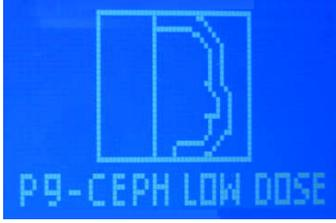
A blue square icon containing a white outline of a human head in profile, facing right. Below the head outline, the text "P9-CEPH LOW DOSE" is written in white, uppercase letters. | <p><b>Low Dosage Digital Cephalometric profile:</b></p> <p>With this profile it is possible to execute a lateral ceph with a smaller exposure area resulting in a lower dose to the patient.</p>                                                                                                 |
