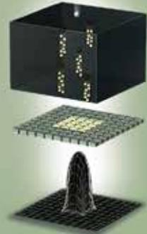
With Panoramic CdTe technology X-rays are not converted to light; therefore, no blurring occurs increasing clarity and contrast.
